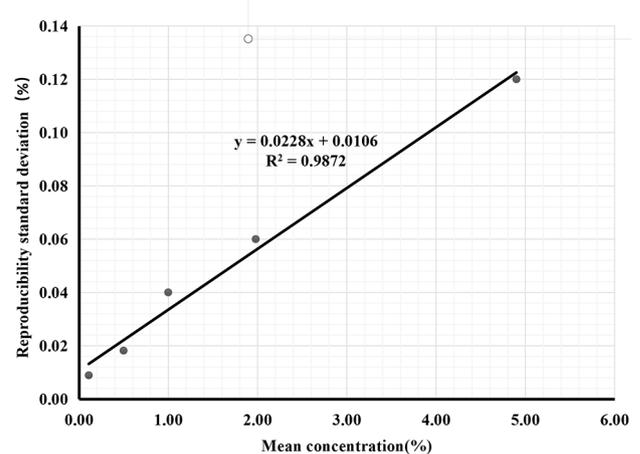
**Fig. 4** Linear regression is produced by plotting mean measurement concentration against reproducibility standard deviation
