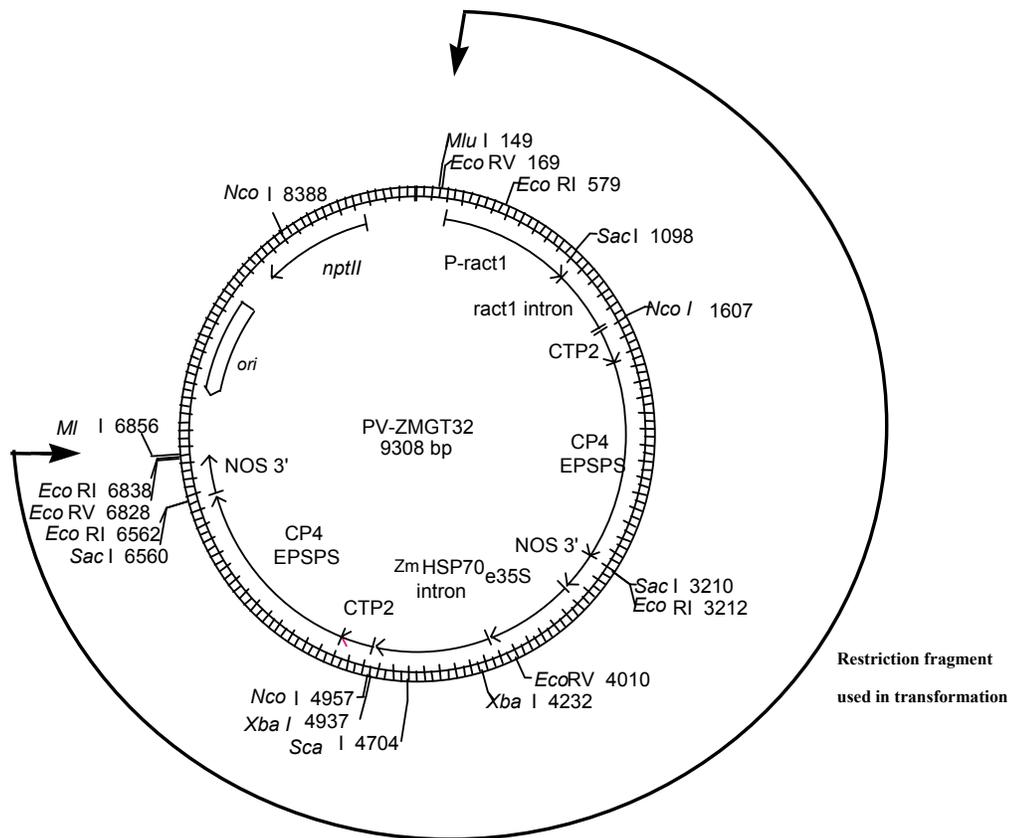
The plasmid PV-ZMGT32 was used to prepare the *Mlu*I fragment used in the transformation of NK603 by excision and discarding of the origin of replication (*ori*) and antibiotic resistance marker (*nptII*) sequences.
